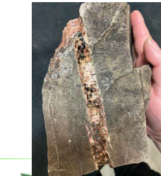
Coarse cassiterite within sub-vertical quartz veins
