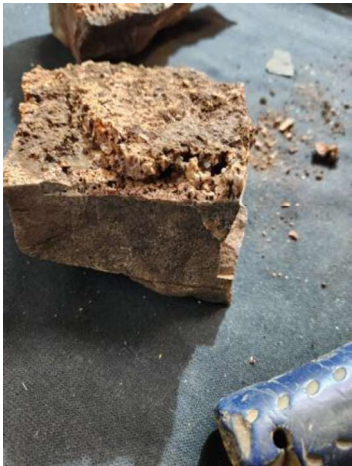
Crushing fractures along quartz veins exposing cassiterite
