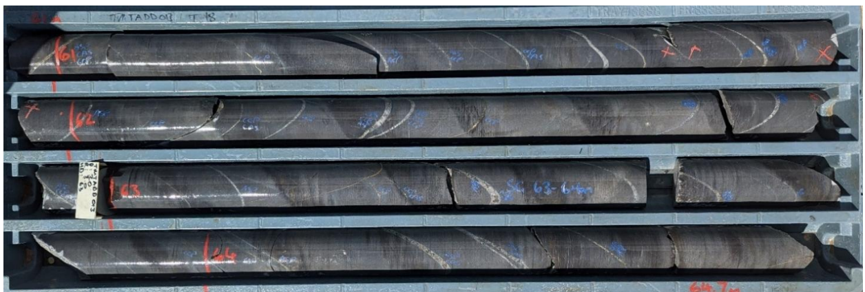
Figure 5-6: North Pit Zone Host Rock and Mineralisation (TMTADD013 61 to 64.7m)
