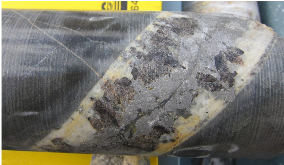
Figure 5-8: Coarse Grained Cassiterite and Arsenopyrite in Quartz Vein (TMTADD001A 126.5m)
