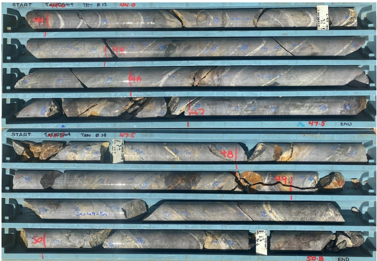
Figure 5-5: South Pit Zone Host Rock and Mineralisation (TMTADD009 44 to 50.8m)
