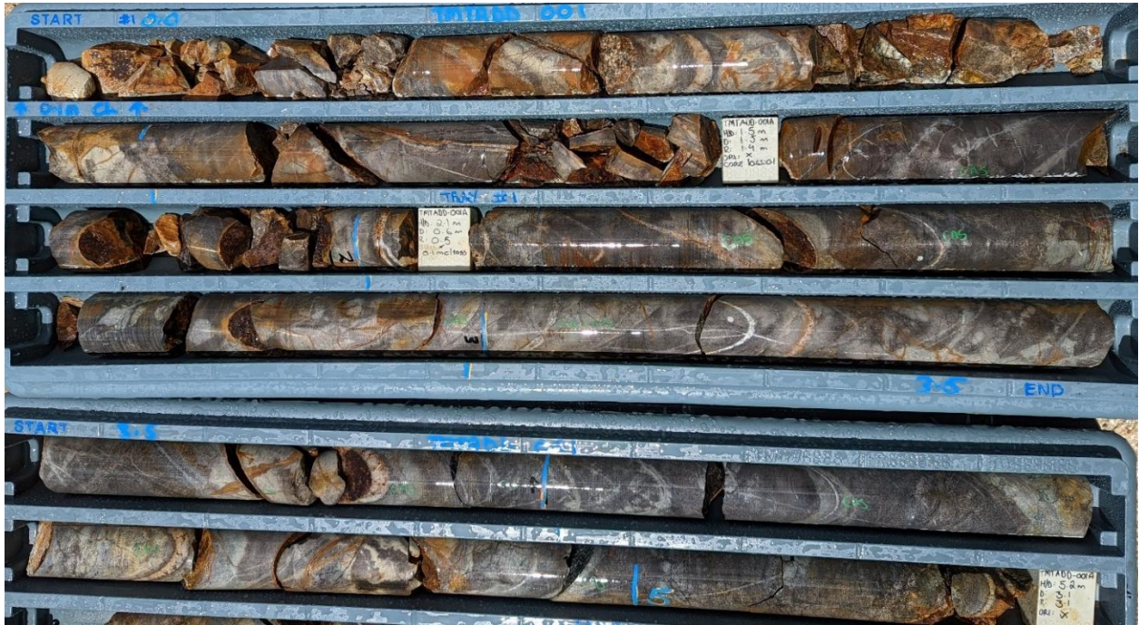
Figure 5-12: An Example of Surface Oxidation from the South Pit Zone (TMTADD001A 0.0-5.2m)
